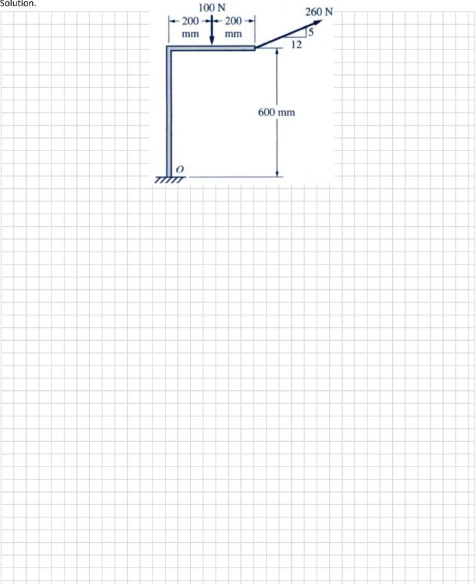
2-43 and 2-44 Determine the resultant moment of the couples acting on the bodies shown in Figs. P2-43 and P2-44. 2-44
